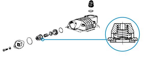
Exclusive stainless steel check valve design ensures perfect sealing performance due to its unique spherical shaped poppet and conical seat.
