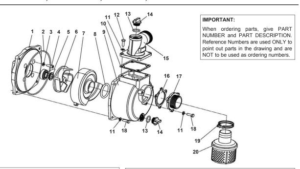
Standard Seal Kit No. 3430-0799 Consists of (1) Ref. 2 O-ring, (4) Ref. 3 Sealed Washers, (1) Ref. 5 Mechanical Seal, (1) Ref. 8 O-ring, (1) Ref. 10 Outlet Sealed Washer, (2) Ref. 13 O-rings, and (1) Ref. 16 Check Valve
