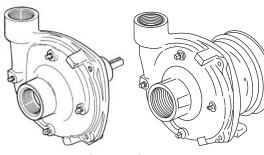
SERIES 9200 Cast Iron, Stainless Steel Pedestal-Mount Centrifugal Pumps
