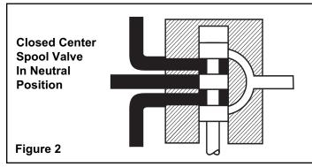
The Closed Center Valve (See Figure 2) is used with variable displacement pumps. The flow is completely shut off in the neutral position, causing the pump stroke to adjust to zero flow. The flow stops, but the pump maintains a static pressure up to the valve.
