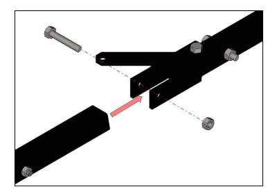
Unscrew Flange Nuts and remove Bolts from hinges on each end of the assembly.
