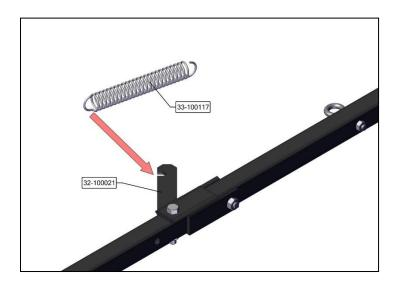
Extend and attach Spring from Boom Eye Bolts to the open holes on the upright portion of the Hinges.
