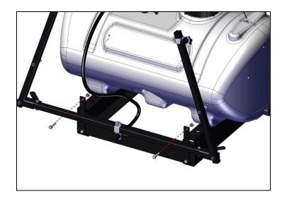
Align Boom Kit holes with open holes on back end of 3-Point Sprayer Frame.
