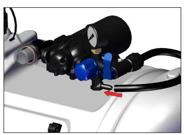
Attach Spray Wand Hose to Elbow Port on bottom of the Regulator Manifold.
