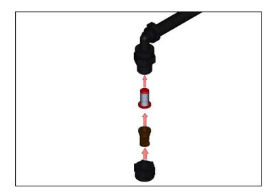
Unthread Nozzle Body Nut and drop Nozzle into Nut for each.
