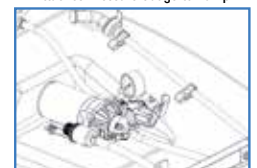
Attaches Pressure Gauge to Pump
