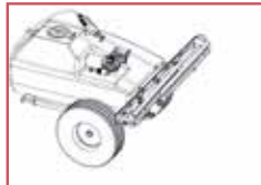
Attached Boom Assembly to Boom Brackets
