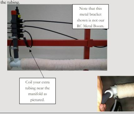
Step #8 Using the weed wiper with your sprayer and installing the electrical wire harness
