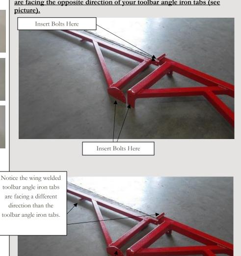
Insert RC Wing pin here
