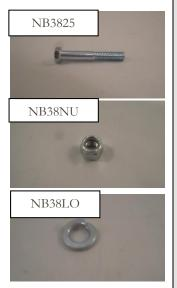
Attach your tank stand (WR1050) to your main frame (WR1000) using the 3/8" x 2 1/2" bolt provided (NB3825 QTY: 1) with the 3/8" lock washer (NB38LO QTY: 1) and 3/8" nut (NB38NU QTY: 1) as pictured.
