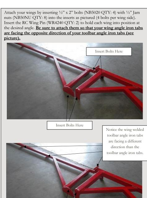
Insert RC Wing pin here
