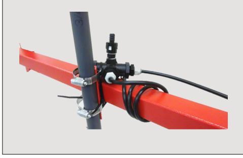
We provide the pump needed to power your weed wiper and the vinyl tubing (VL0038 QTY: 15 ft.) needed to run from your manifold to your pump (since your manifold has been mounted to the center of the boom). Use our CL0916 clamps to secure your tubing to your manifold and pump. Any extra 3/8" tubing may be coiled up. Now, connect your manifold inlet to your spray pump as pictured.
