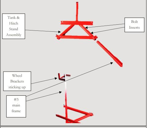
Bolt your rear tool bar (#4 in diagram) to the back of your left frame (#2) and your right frame (#3) with 3/8" x 3" (NB3830 QTY 6) bolts (with the 3/8" lock washers (NB38LO QTY: 6) & 3/8" nuts (NB38NU QTY: 6) on <u>each side</u> using the inside holes. Make sure that the angled iron brackets pictured below are facing toward the front of your weed wiper model (i.e. towards the front hitch)
